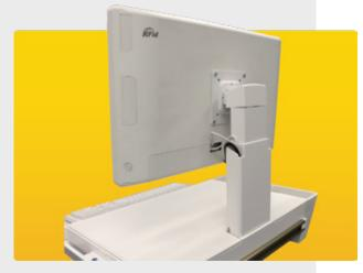
Cables to the AIO can be easily routed making it tidy and easily to clean.
